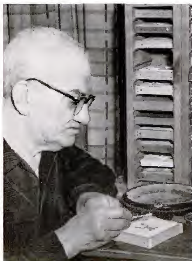
Riddle ladles rubber solution into a mold to make a little green frog. After pouring, he sets the mold aside for eight hours so that the rubber can cure
